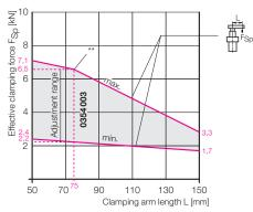
\*\* For clamping arm lengths > 75 mm, please observe the setting parameters permitted for the effective clamping force as specified in the operating instructions.
