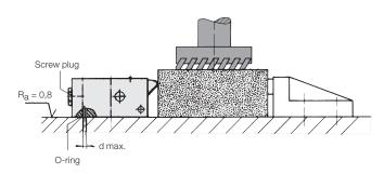
The hydraulic oil can optionally by supplied through tubes or drilled channels in the fixture body; 4 fixing screws are required.
