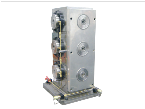
SPEEDY classic 1 fast closing clamp fitted to each side of a mounting tower with pipework, protected by cover plate (one side without cover plate so that the pipework can be seen)
