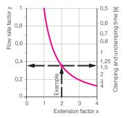
Adm. flow rate and clamping time as a function of the clamping arm extension
