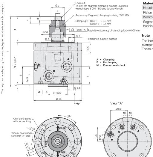
Only bore clamp with compensation in direction of arrow
