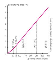
Friction value  $\mu$ = 0.1 (steel / steel dry) between centring cone and segment clamping bushing. With lubrication, the expansion force can double!
