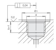
Sealing is attained by a knife edge at cylinder collar, requiring the sealing surface to be square to hole axis and flat.
