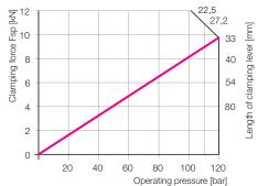
Example 1: Flat lever clamp 1829423D24 Operating pressure 100 bar Standard clamping lever L = 24 mm
