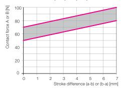
Diagram valid for horizontal mounting position. For vertical arrangement the weight of the clamping jaws has to be considered.
