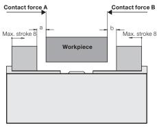
**Limit dimensions:** a max. = 7 mm b max. = 7 mm
