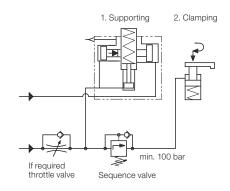
The sequence valve has to be adjusted to an opening pressure above the intersection of the two straight lines in the diagram.
