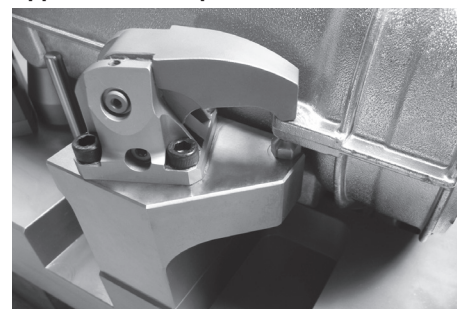
Clamping of a cast part
