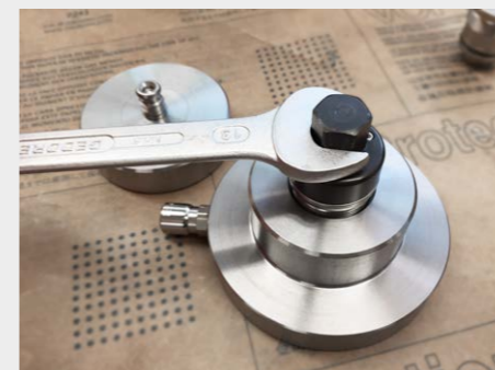
Tighten with mounting key (15 Nm)
