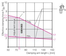
\*\* For clamping arm lengths > 75 mm, please observe the setting parameters permitted for the effective clamping force as specified in the operating instructions.
