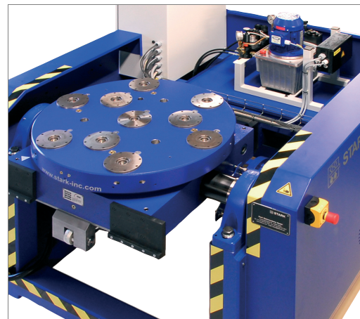
SPEEDY classic 2 fast closing clamps, fitted in round plate on setup station.
