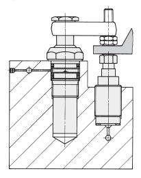
Support and clamping forces have to be adapted to each other, so that there will be sufficient force reserve available for the threaded-body work support to absorb the machining forces.
