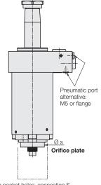
With pocket holes, connection S can be used for venting
