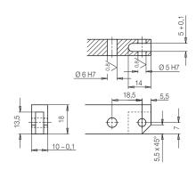
Example 1: Hinge clamps 1826011 Operating pressure 60 bar Standard clamping lever L = 22 mm
