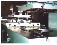
Double-T clamping bar on press bed and ram
