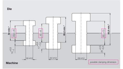
\* Minimum slot dimension when using double-T clamping bars without carrying rollers, height in unclamped condition +0,5 mm (= d max. -c + 0.5)
