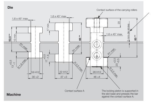
Note: The die stroke of 2 mm is exemplary (e.g. for larger die stroke, reduce the slot depth accordingly).
