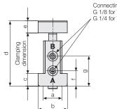
Connecting thread on both ends G 1/8 for T-slot 18 G 1/4 for T-slots 22 and 28
