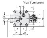
Bore hole for plug-in check valve
