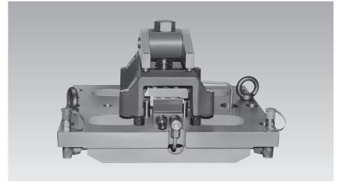
The opposite figure shows a hydraulicallyoperated fixture for concentric positioning and clamping of two casted housings, whose interior surfaces are due to functional reasons have to be concentrically arranged to the machined holes.
