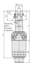
A = Clamping **B** = Unclamping
