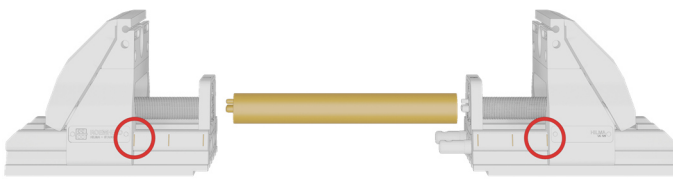
Fig. 41: Inserting the adjusting spindle extension
