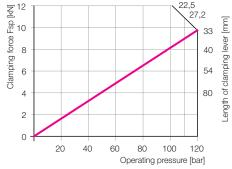
Example 1: Flat lever clamp 1829423D24 Operating pressure 100 bar Standard clamping lever L = 24 mm
