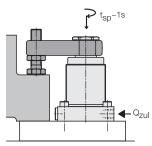
Longer special clamping arms are heavier and have a higher moment of inertia.
