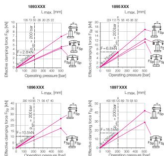
\*) In the case of single-acting swing clamps, the spring force has to be considered.
