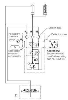
Power unit with a pressure filter 10 µm is required.
